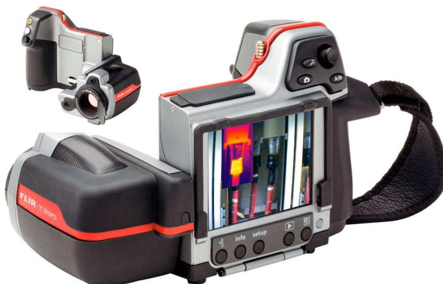
Obr.9. Termokamera Flir T335 [39]
