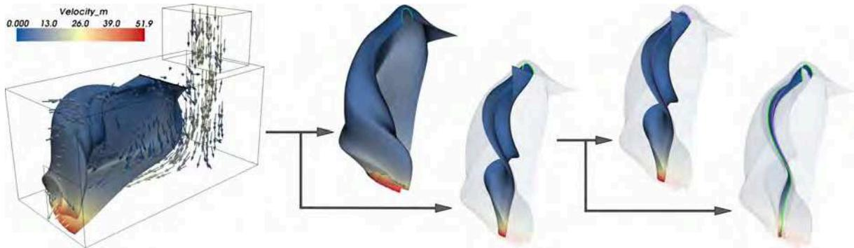
Figure 8: CFD simulation of a fluid flow in a box. The leftmost picture gives an overview of the dataset with the extracted stream surface. The other pictures show the surface after the first and the second cut.
