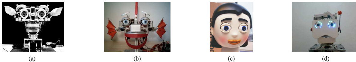
Figure 1: Robot heads designed in hardware: (a) Robot head “Kismet”, Breazeal et al. [Bre99, Bre03], (b) Emotional-display “EDDIE”, Sosnowski et al. [Sos06], (c) Cartoon-like robot head “Flobi”, Lütkebohle et al. [Lüt10], (d) Head of general-purpose social robot “Bender”, Ruiz-del-Solar et al. [Rui09].
