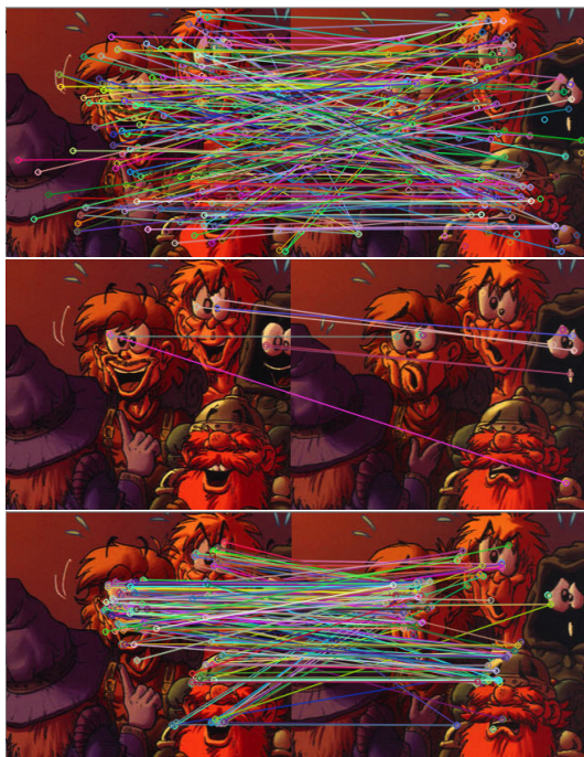
Figure 8: Up to down: SIFT, SURF and ORB detectors on ROI of two panels of comic Le Donjon de Naheulbeuk .
