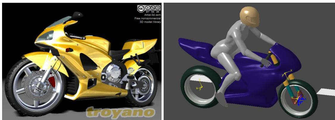
Figure 6-54 – a) Original PTW model (artist-3d.com); b) Human model in Virtual.Lab with helmet, in a PTW and road scenario.
