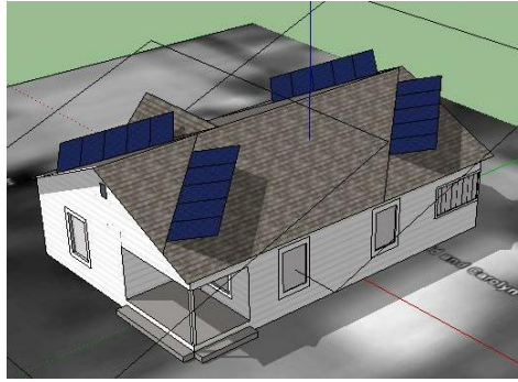
Figure 20: Solar panels on a slightly inclined roof [12]
