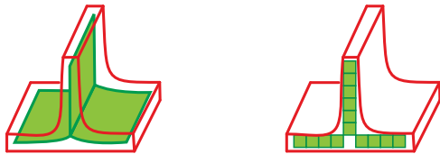
Figure 1: An example of medial surfaces(left) and medial voxels(right)
