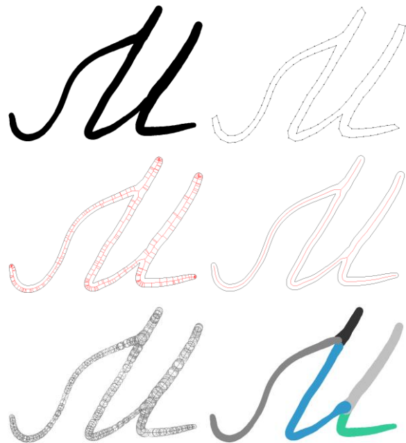
Figure 7. The transformation of the raster character to the set of fat curves.
