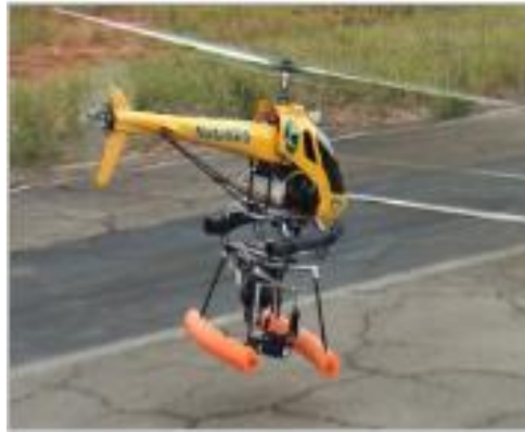
Figure 2: Our small helicopter with the pan-tilt image and video acquisition head
