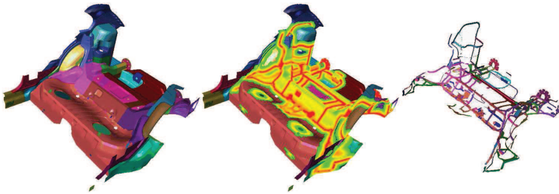
Figure 10: These images show parts of the back compartment of a car. The illustration in the middle visualizes the minimum distance from each node to the closest surface of another car body part up to 50 mm. On the right the same values are mapped to hide all geometry where this distance is more than 2 mm using the texture subsystem and the alpha test. The rendered geometry show potential flanges.
