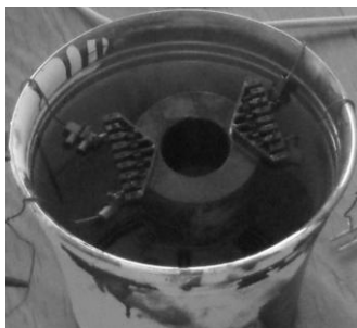
Fig. 1. Measurement transformer without magnetic liquid
