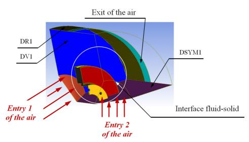
Fig. 4. Definition of surfaces of the fluid field
