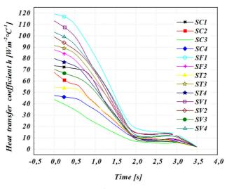
Fig. 10. Variation of the heat transfer coefficient h for various surfaces of the full disc in a transient case (FG 15)
