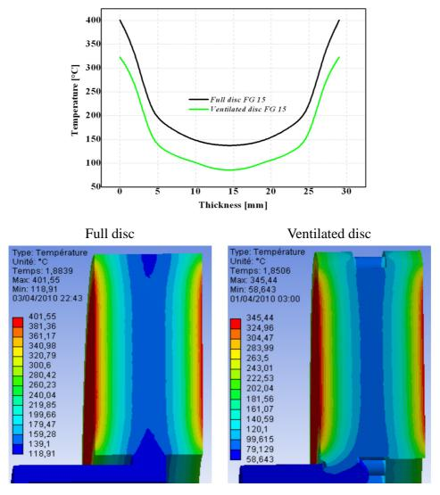
Fig. 18. Temperature variation through the thickness for both designs of the same material (FG 15)
