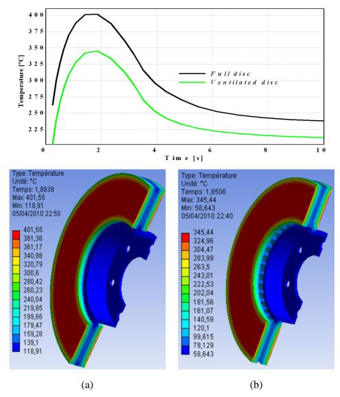
Fig. 16. Temperature distribution of a full (a) and ventilated disc (b) of cast iron (FG 15)
