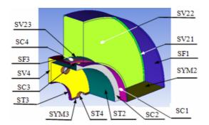
Fig. 8. Definition of surfaces of the full disc
