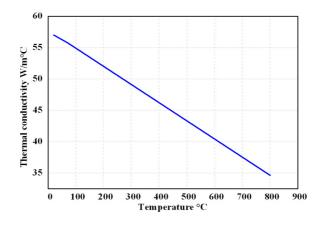
Fig. 2. Thermal conductivity versus temperature
