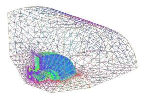
Fig. 5. Mesh of the fluid field
