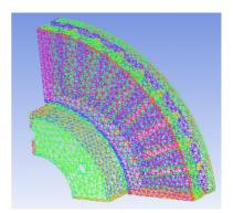
Fig. 6. Mesh of the full disc (Number of elements 272 392)
