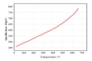
Fig. 3. Specific heat versus temperature
