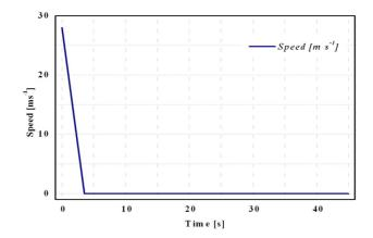
Fig. 12. Speed of the vehicle versus time (braking of type 0)
