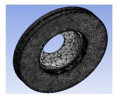
Fig. 15. Ventilated type disc mesh model (total number of nodes 154 679 — total number of elements 94 117)
