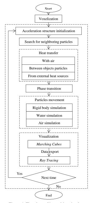
Figure 1. Flowchart of ice melting simulator
