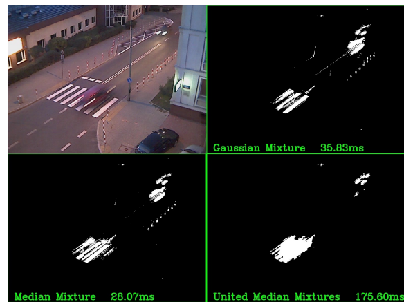
Figure 5. Comparison of all three methods in an extreme situation – lots of reflections, from top left: input image, the results of the GMM, the results of the MMM, the results of the UMM.
