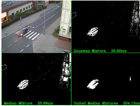
Figure 6. Comparison of all three methods in extreme situations – sudden light change, from top left: input image, the results of the GMM, the results of the MMM, the results of the UMM.
