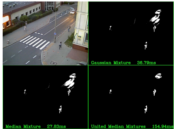
Figure 8. Comparison of all three methods in extreme situations – reflection and 3 people, from top left: input image, the results of the GMM, the results of the MMM, the results of the UMM.
