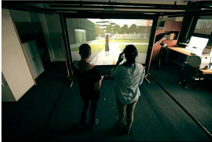
Fig. 1. Target single-screen CAVE with IS-900 tracking device
