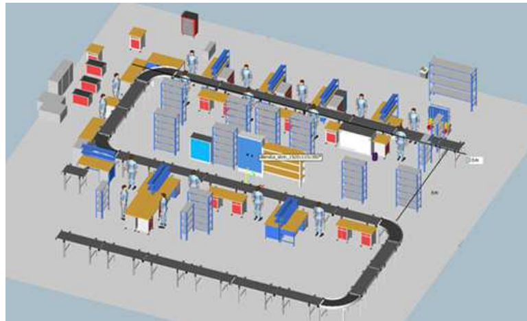
Fig. 2. Manufacturing layout of a reference model (in Siemens NX)
