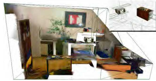
Figure 11: Confined space ( 9 m^2 ) home office scene: 3D view of extracted textures from light probe and detail perspective images.
