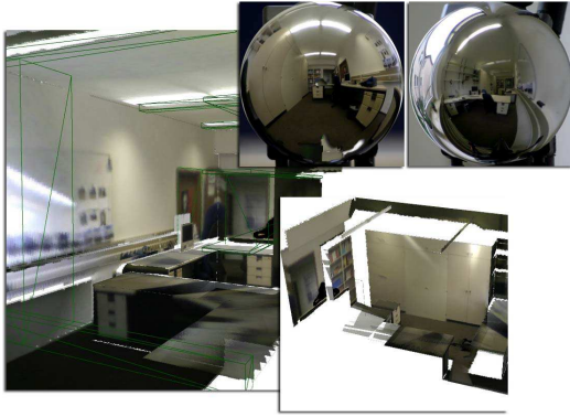
Figure 9: Reconstruction of a small office from two light probes with 800x800 pixels each. This example shows the projection of an unmodelled chair onto the desktop.
