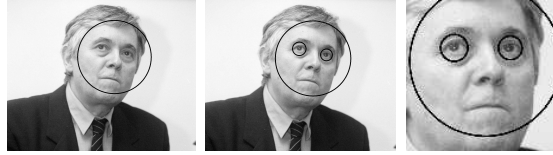
Figure 4.4: Example of face detection (left), eye detection (middle) and face rotation according to the eyes (right)
