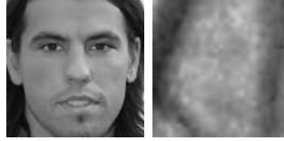
Figure 4.1: Example of one correctly detected face (left) and one incorrectly detected face by the Viola-Jones face detector
