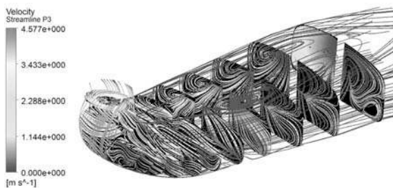
Fig. 14. Skin friction lines and surface streamlines in case of DFT-A
