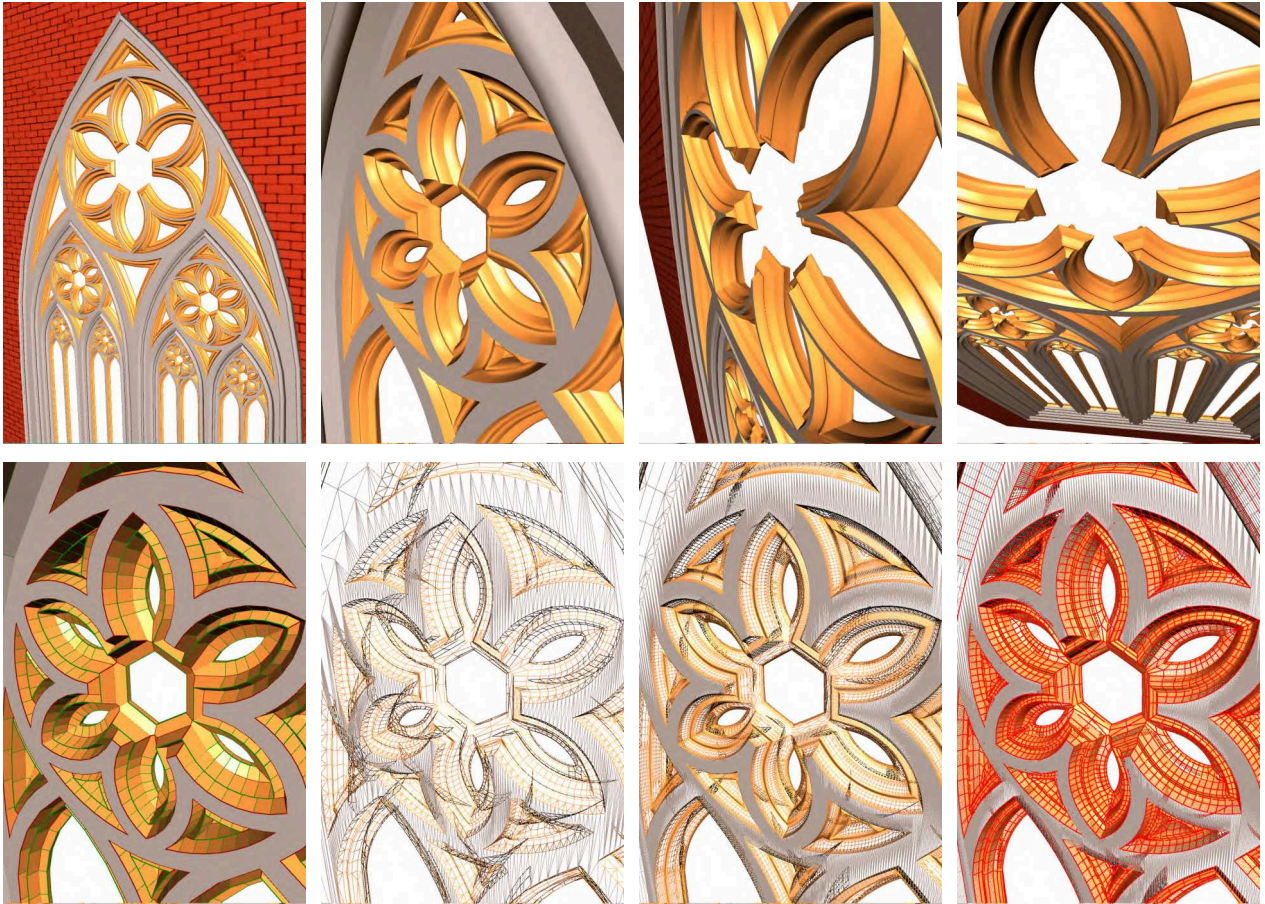
Figure 12: The top row shows images from the Gothic Window animation discussed in Section 6.3. The bottom row show the polygonal B-rep mesh, and subdivision surface tessellations in low and high resolution, and also the individual patches.
