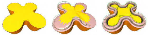
Figure 7: Motivation for Euler macros. The center image shows an intermediate configuration from the construction of a profile (right). In order to avoid such inconsistent LODs, all operations leading from one consistent state to the next can be grouped into one Euler macro.
