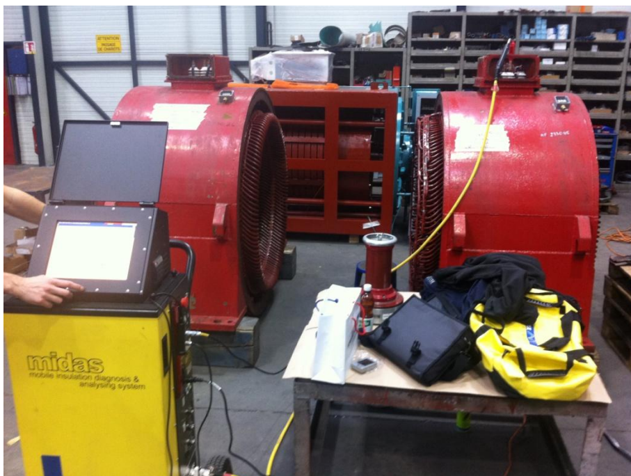
Fig. 87 Stator winding U_n = 5.5 kV.
