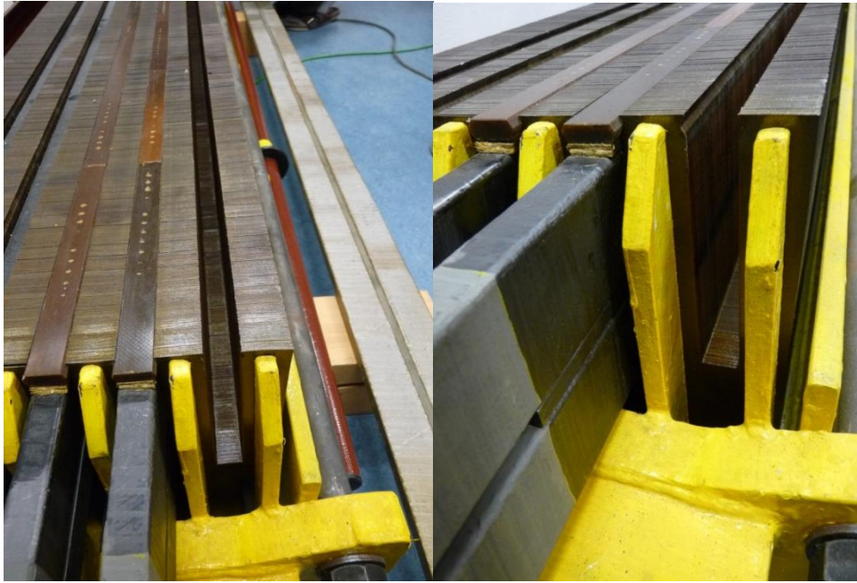
Fig. 19 Tested model of rotating machines stator winding
