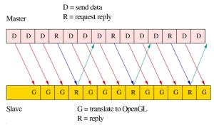
Figure 3. Asynchronous reply mechanism.
