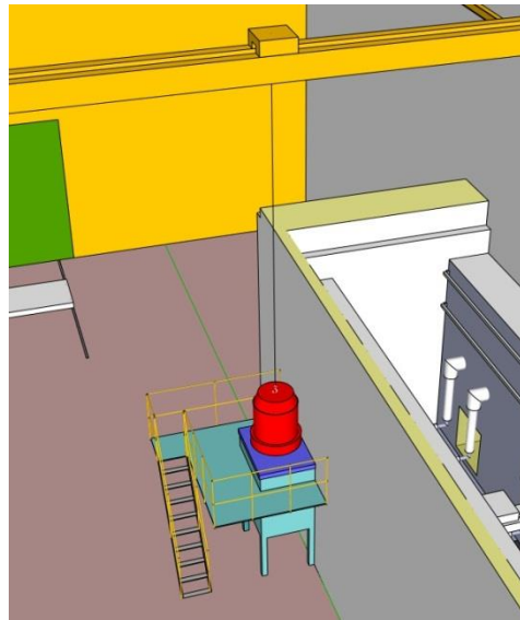
Figure 14 The shielded cask on the input chapel
