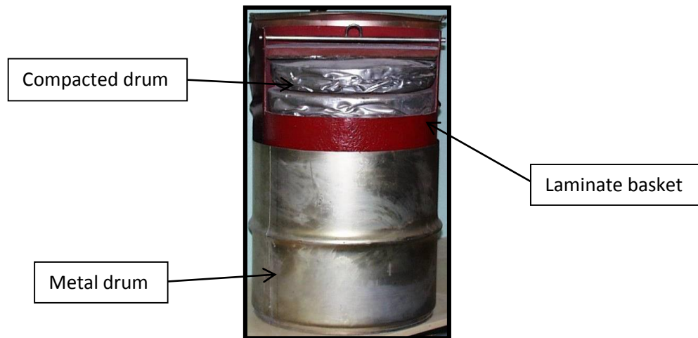
Figure 11 The drum with the waste [4]
