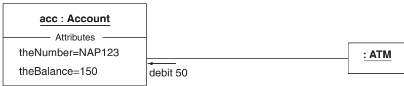
Figure 1.6 Message from an ATM to an account object
