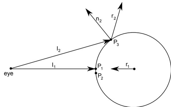
Figure 4: Incident and corresponding reflected vectors
