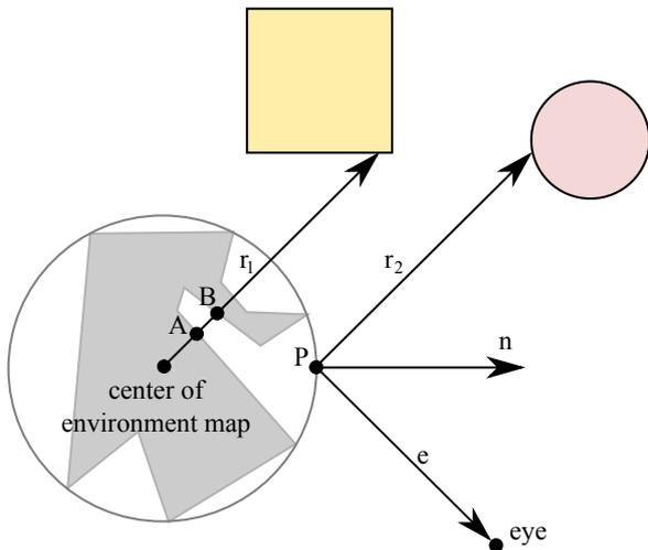
Figure 3: Environment mapping has two major problems: First of all each reflection is computed as if the reflecting point ( $P$ ) would lie in the center of the environment map. Also it cannot handle self-reflections, which leads to incorrect shading results at point A.
