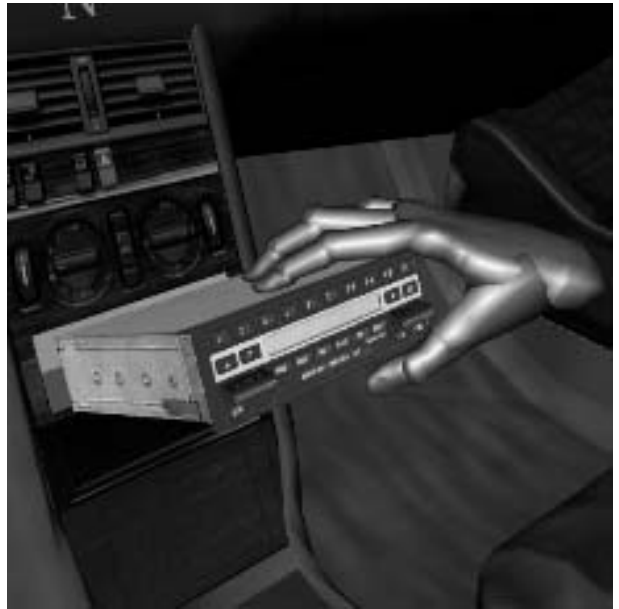
Figure 3: Ergonomy study and assembly simulation in a virtual car interior. The user has to install the car radio.
