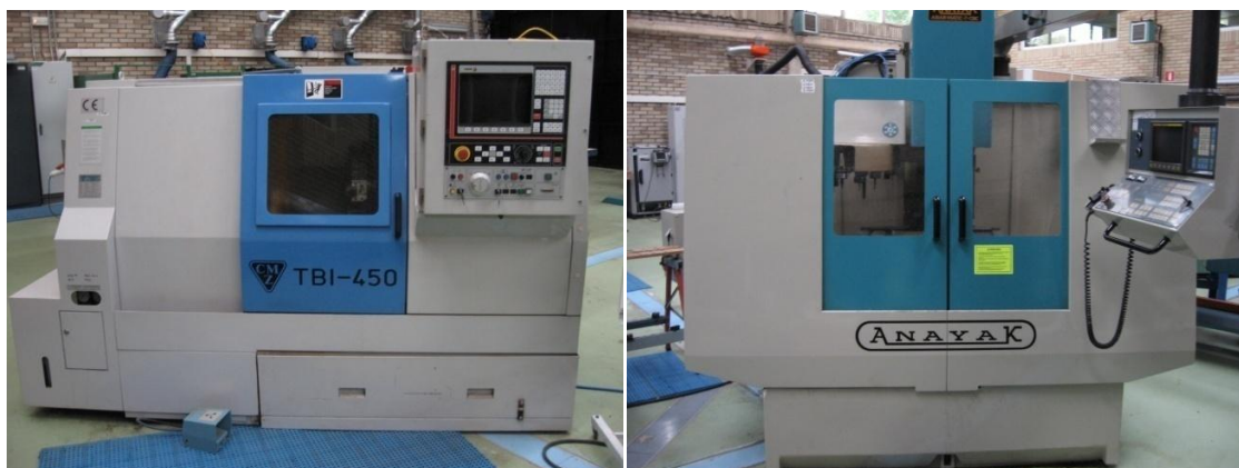
Fig. 5: Machines, where manufacturing was made (left: lathe CMZ TBI - 450; Milling centre ANAYAK ANAK-MATIC-7-CNC)
