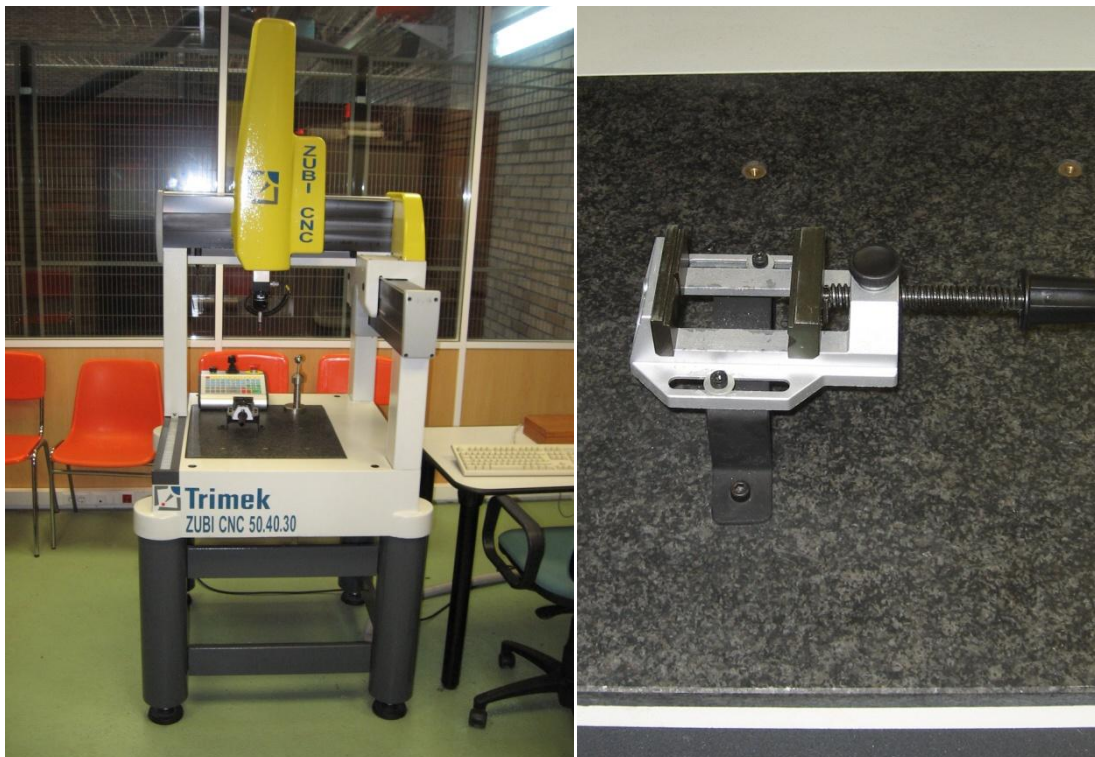
Fig. 1: 3axis measuring machine Trimek (right side: detail of improvised fixing of vice)
