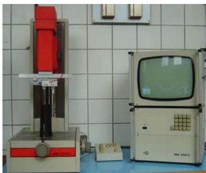
Figure 3: Measuring device MK 300C and profiles measured for components
