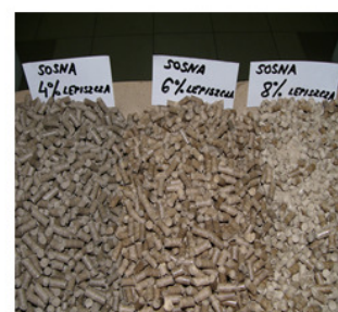
The effect of different binders on stability of the pellets
