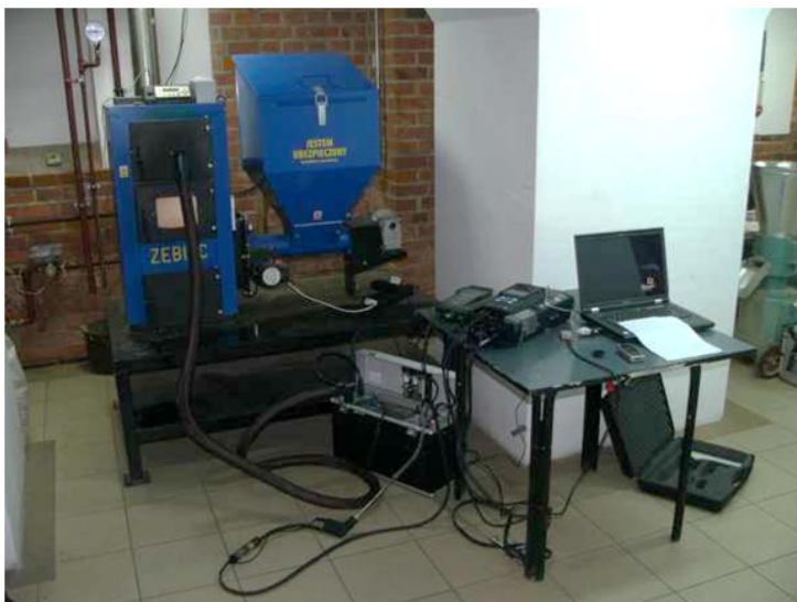
Investigation of the content of gas pollutants in flue gases ( O_2 , CO, NO, HCl, VOCs) – the retort boiler 15kW
