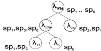
Figure 3.: Regression tree for 6 speakers, sp\_i is the speaker i and \lambda_{ij} is the model for the speaker i, jj
