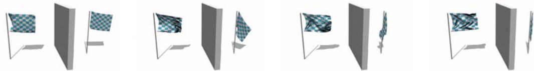
Figure 5: Two flags blowing in the wind (particle tracing method). The wind is blocked by the wall, so the right flag is in the lee (compare figure 4).
