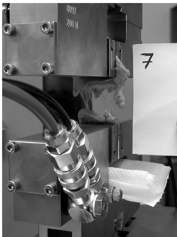
(a) Heart valve tissue sample between the pneumatic grips of the 200 N loading cell of the experimental apparatus Zwick Roell Z050.
