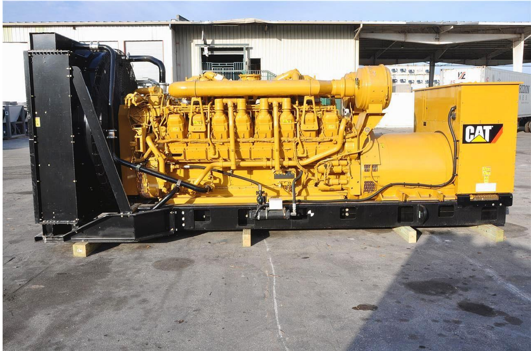
Obr. 11 Dieselagregát CAT 3516B HD [17]
