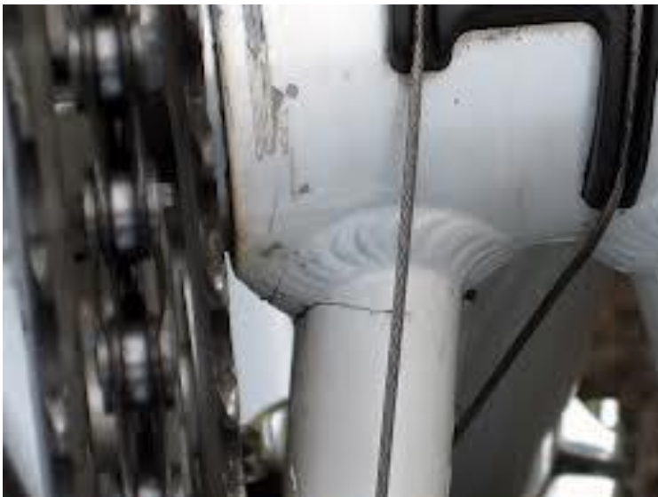
Prasklina rámu [27] zdroj: https://encryptedtbn1.gstatic.com/images?q=tbn:ANd9GcQERnG0HjbNerBKwNiemTbBsBRq0AbE55Dc1YzDWh_z5tUuhDBIwg
