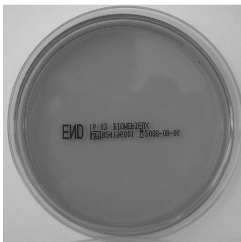
Figure 5.1.8. Picture illustrating strong killing efficiency of Escherichia coli bacteria exposed to UV irradiation on TiO 2 /Cu film surface where the irradiation was followed by cultivation for 24 h at 37°C on Endo agar covering the Petri dish.
