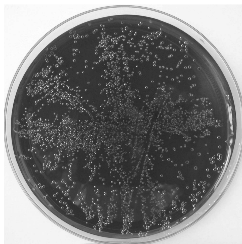
Figure 5.1.6. Picture illustrating very weak killing efficiency of Escherichia coli bacteria exposed to UV irradiation on TiO 2 /Cu or TiO 2 film surface where the irradiation was followed by cultivation for 24 h at 37°C on Endo agar covering the Petri dish.
