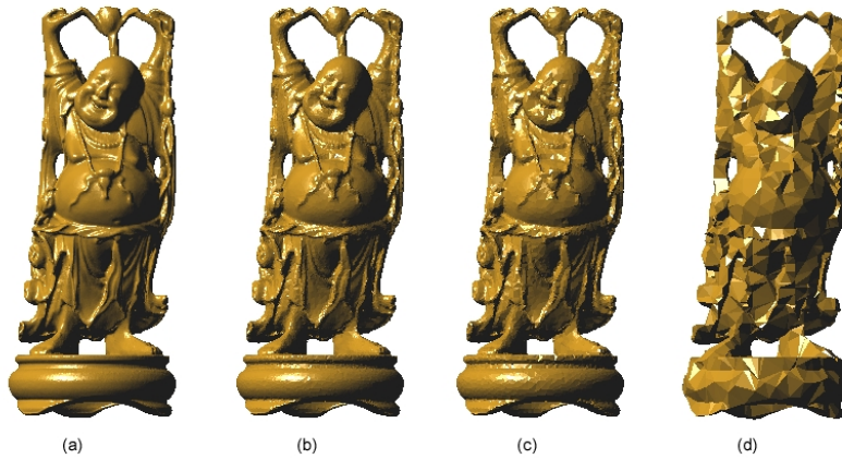
Figure 14: The Happyb model (courtesy GaTech) at different resolutions; the original model with 1,087,716 triangles (a), reduced to 105,588 triangles (b), 52,586 triangles (c), 10,974 triangles (d)
