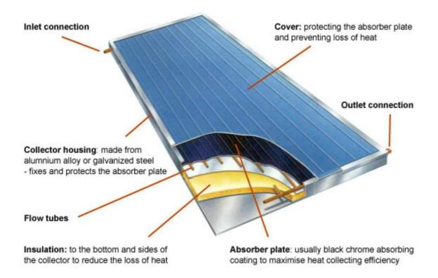
Figure 2 – Flat plate collector [3]
