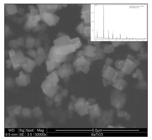
Figure 1 – Crystals of barium titanate prepared in hydroxide melt On inset is crystal structure from XRD measurement
