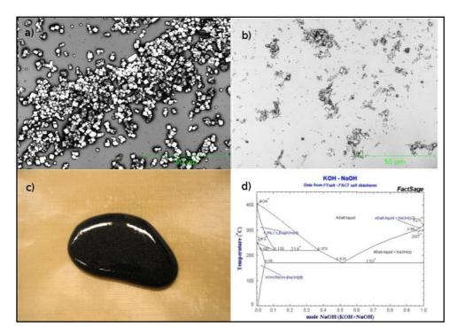
Figure 2 – a) PbTe cubes with laser confocal microscopy, b) CuS rods with laser confical microscopy, d) Black PbS in eutectic hydroxides on Teflon foil, d) Eutectic diagram of NaOH and KOH
