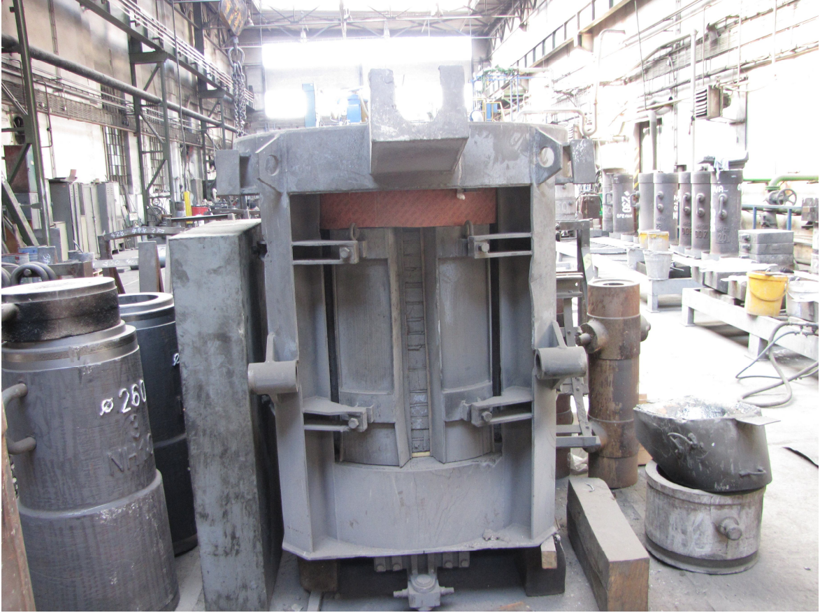
Figure 2 – Sample inductor separated from the vacuum induction crucible furnace (1000 Hz, 1000 kg) with shielding transformer plates bunches
