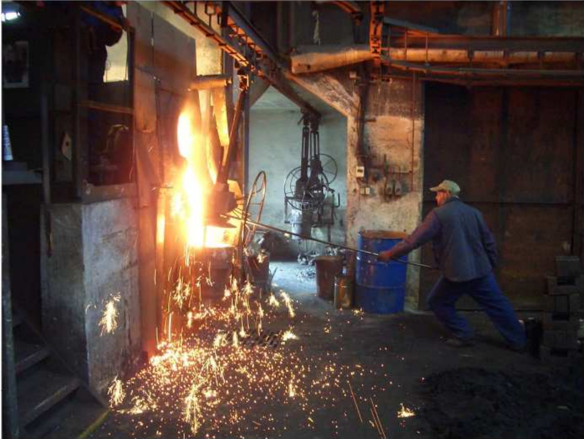
Figure 2 – Outpour of the furnace
