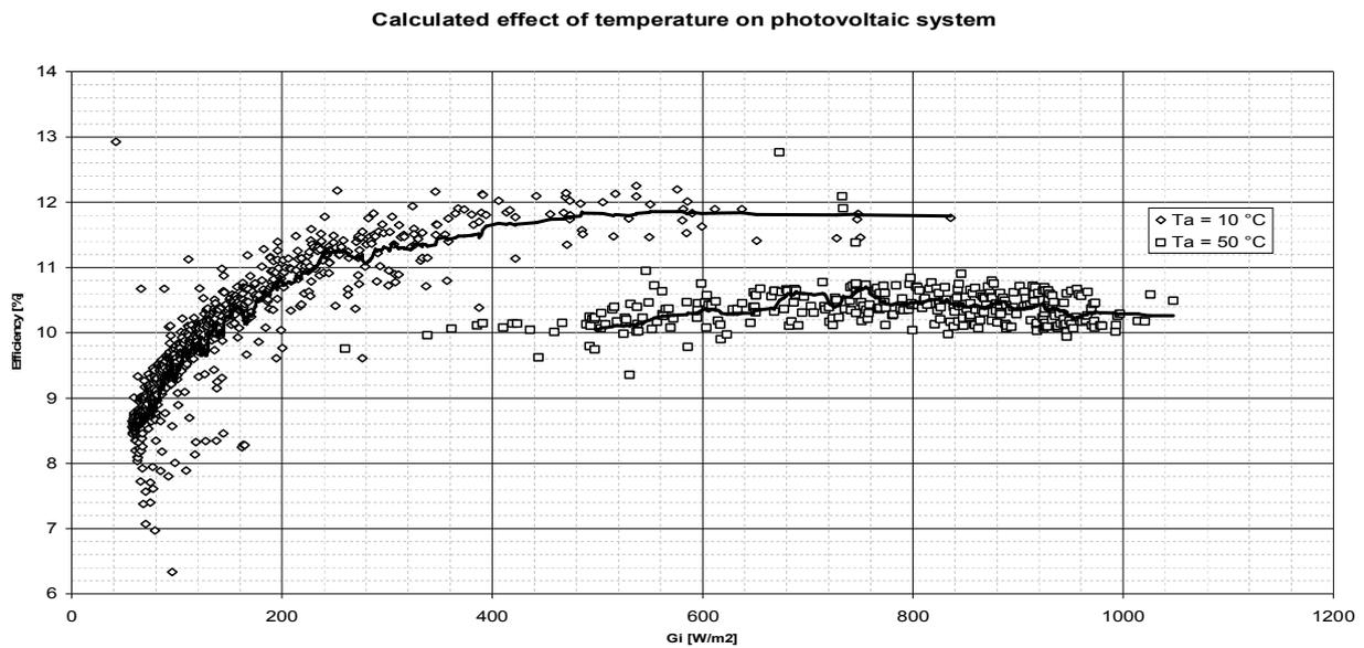
Chart 3 – Calculated effect of temperature on photovoltaic system
