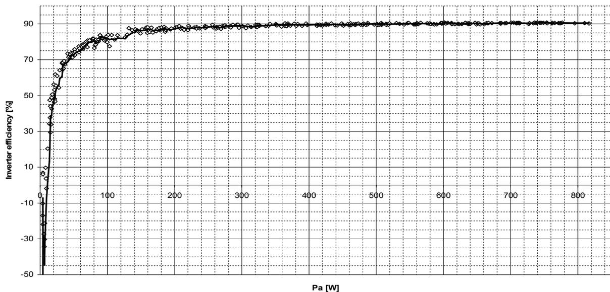
Chart 1 – Measured inverter efficiency
