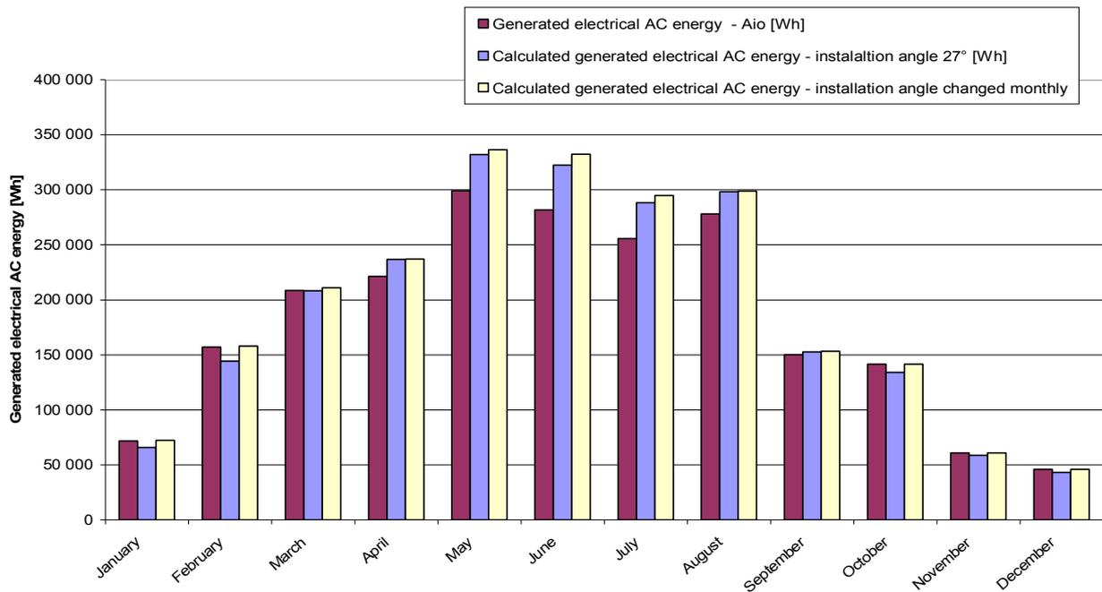
Chart 2 – Measured and calculated generated electrical AC energy
