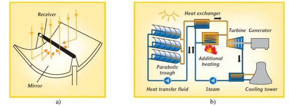
Fig.1. a) parabolic mirrors focus the sun's rays onto the receivers b) Diagram of the parabolic trough power plant [3]
