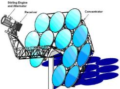
Fig. 2. Schematics of a dish/engine system with stretches/membrane mirrors. [4]
