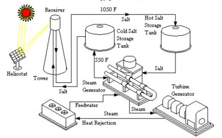
Fig.3. Schema of Solar Power Towers [5]
