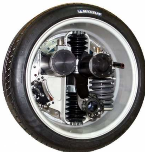
Obr. 19. Michelin Active Wheel 19
