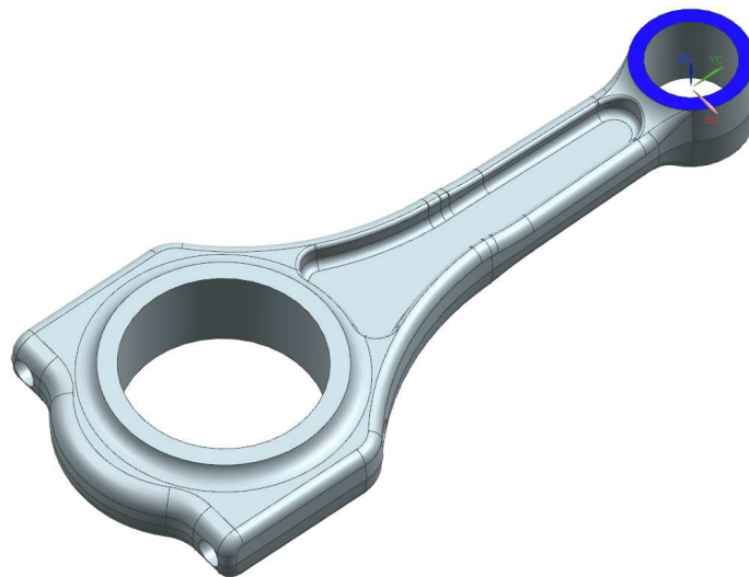
Figure 69 – Simplified geometry of the connection rod
