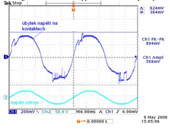
Fig.4 Voltage characteristic on the surface layers in the electrical contact
