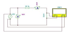
Fig.3. Wiring diagram of electric contact measurement
