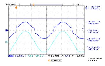
Fig.5. Voltage characteristic on the surface layers in the electrical contact
