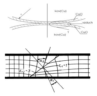
Fig. 2 .: Stationary contact with thin alien film, Settlement of two dielectric with different absolute permittivity [4]
