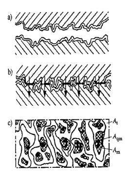
Fig. 1. Stationary contact with thin alien film, [1]
