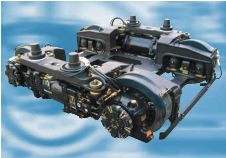
Obr. 9: Podvozek Combino SF 30C TFW [3]
