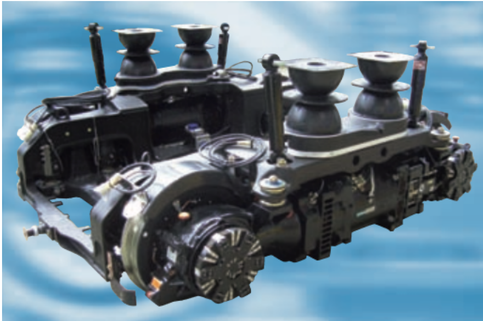
Obr. 10: Podvozek Combino SF30C TFW/LFW [3]
