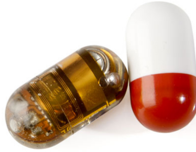
Fig. 1.3: BodyCap e-Celsius ® is a miniature electronic pill that monitors and communicates wirelessly the intracorporal temperature.
