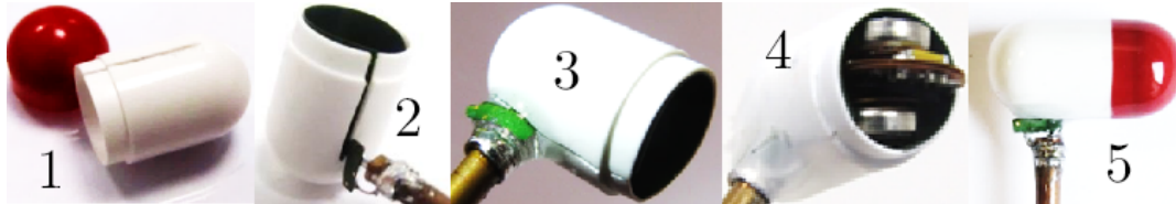
Fig. 4.21: Capsule preparation process for the impedance measurement: 1) to cut the PVC shell; 2) to insert the antenna and to measure the impedance; 3) to fix the connection with the epoxy resin for the mechanical rigidity and to re-measure the impedance; 4) to insert the capsule circuitry and to fill the capsule with the epoxy; 5) to measure the capsule impedance after 24 h (epoxy curing time).
