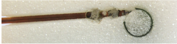
Fig. 4.20: Conformal antenna in the Rohacell IG 51 foam ( \epsilon_r = 1.05 , \tan \delta = 0.0003 ).
