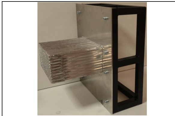
Figure 3: Attenuator as Constructed
