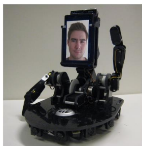
Figure 5. A robotic platform for socially embodied telepresence was presented by [Ada10a].
