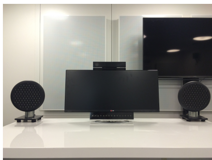
Figure 2: Hardware prototype of the presented acoustic interface, consisting of the Kinect 2 depth sensor, a 13 channel microphone array, and two parametric arrays mounted on automatic alignment units.
