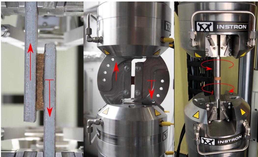
Figure 2 – Shear and torsion tests
